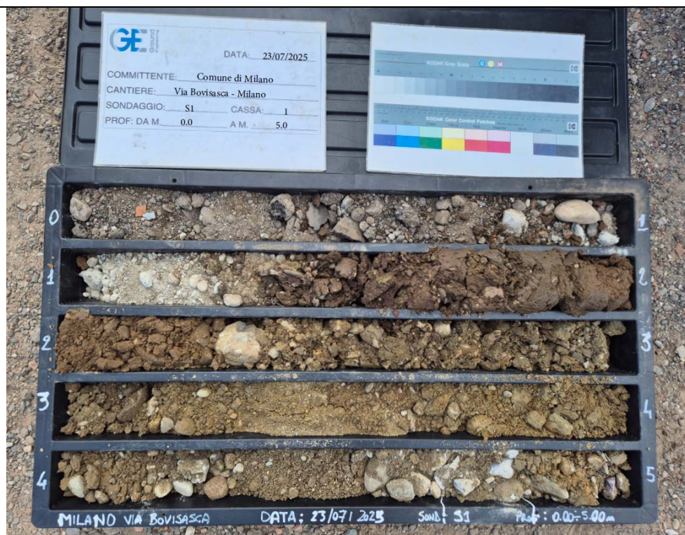
SONDAGGIO S1 – CASSA 1 – DA 0,0 A 5,0 M
